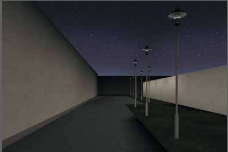
Skyline 150w CDM-TT mounted on 4m columns at 6m centres
