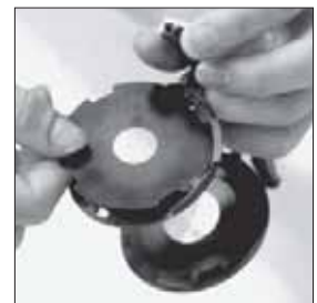
Interchangeable irises in three sizes
