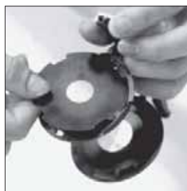
Interchangeable irises in three sizes
